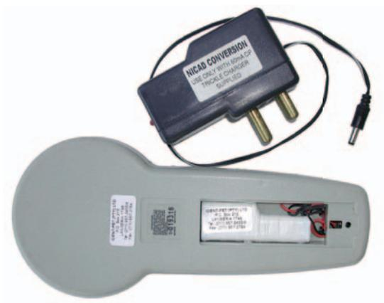
The Pocket Reader EX is powered by a rechargeable battery pack.
